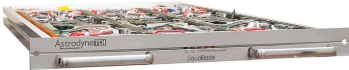
Providing high operating efficiency along with excellent reliability, compact size, and easy maintainability; LiquaBlade™ power supplies are the ideal choice for high power DC systems in industrial and military applications. The converter features automatic load sharing and international power input.
