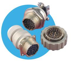
**Mk18 (Pattern 608).** A complete system of medium density connectors and accessories designed to withstand extreme environmental conditions. Meeting the requirements of BS9522-F0020, Mk18 connectors are particularly suitable for exposed areas in marine and land based equipments. The nickel aluminium bronze shells provide excellent corrosion resistance coupled with high strength.
