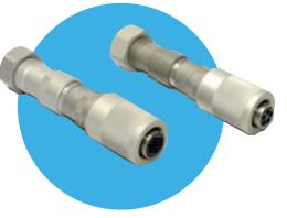
**Mk22.** Low to medium density connectors with sealed cable outlets designed for marine applications. Materials, finishes and construction have been engineered to meet the severe environmental and mechanical demands encountered in above and below deck applications. MK22 connectors are approved to VG96930 specification.
