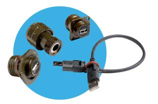
The high speed **RJ45 & USB** connector systems incorporate an ABAC (MILDTL-38999 series III) or AB05 (MIL-DTL-26482) derived metal shell with full 360 degree EMC and mechanical protection, and has been designed to meet the requirements of high speed data connections where reliability through environmental sealing and enhanced mechanical protection are required.
