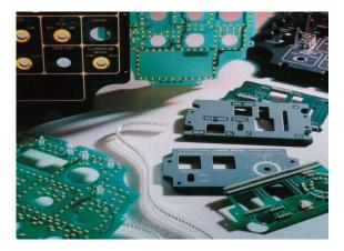
The choice of LED's in a Surface Mount configuration enables panels for Aerospace and Military applications to be manufactured in accordance with the requirements of MIL-DTL-7788 (Formally SAE AS7788) for Type VII panels.
